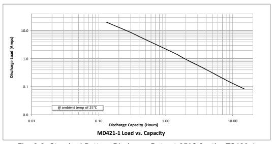
Fig. 3.3 Standard Battery Discharge Rate at 25°C for the TS420-1
