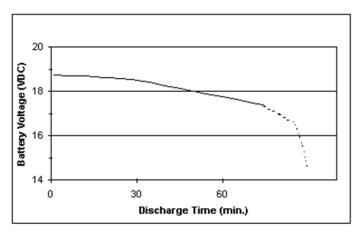
Fig. 3.1 Nominal Battery Discharge Rate at 20°C for the TS420 used with Mid Continent Instruments 4200/4300 Attitude Indicator
