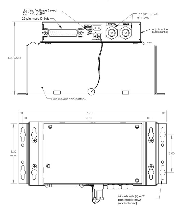
Figure 2.2 MD421-1 Battery Module Mounting Dimensions
