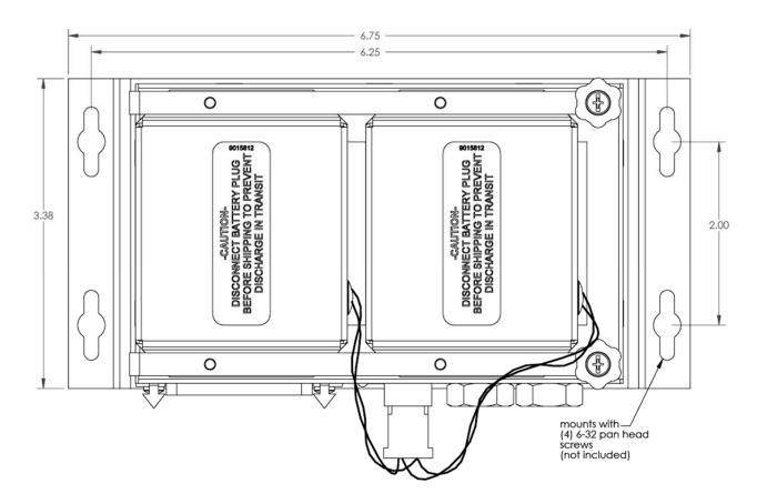
Figure 2.1 MD421 Battery Module Mounting Dimensions
