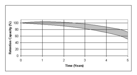
Fig. 3.5: Life Characteristics In Standby Use
